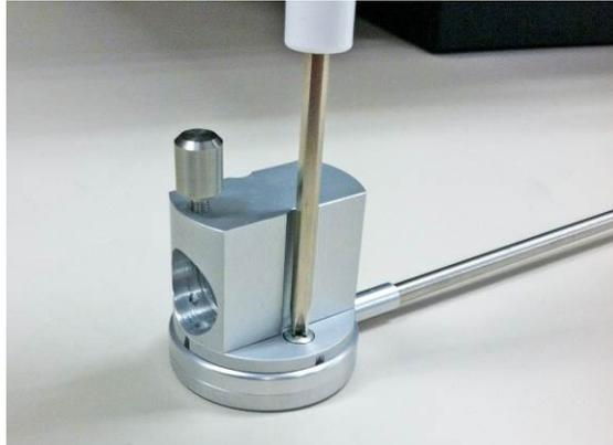
3. Insert the LED Wand into the Optic Adapter until it bottoms out. Tighten the set screw on the top of the Optic Adapter when the LED Wand is installed.
