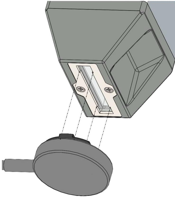
**Figure 14. Adapter Alignment**
