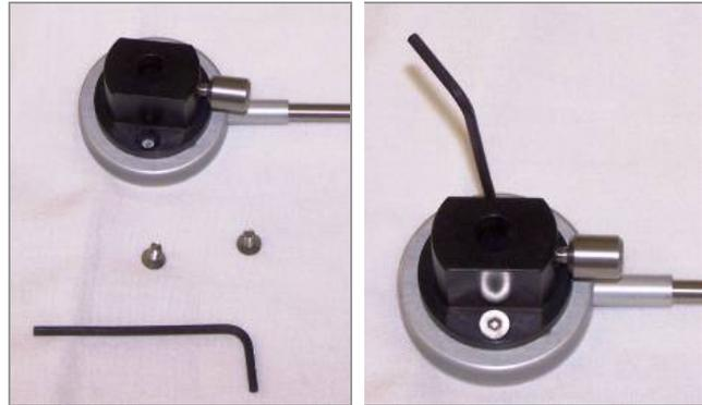
4. Insert the lightguide into the lightguide adapter until it bottoms out. Tighten the set screw when the lightguide is installed.
