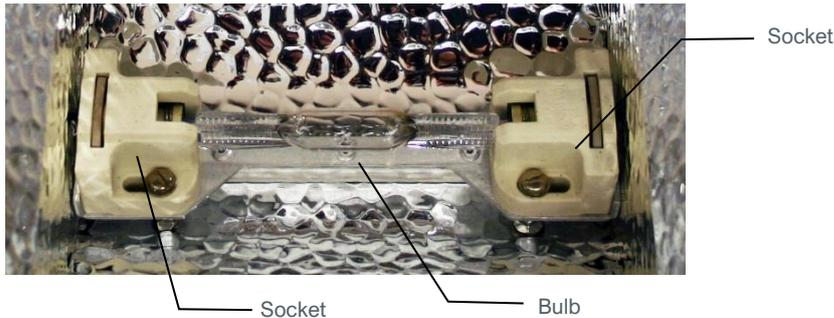
Step 5. Lightly push the Bulb toward the Socket on the opposite end of the lamp so that the end being grasped can be lifted clear of the Socket.
