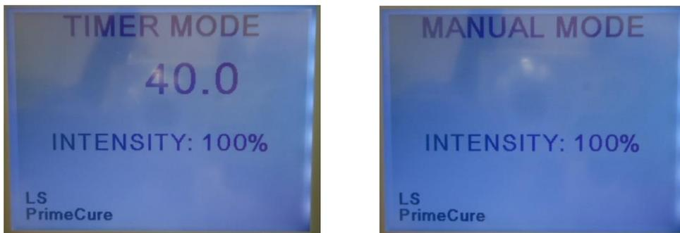
**NOTE:** If your unit doesn't display the 'LS' symbol on the screen, remove all power and do not operate the unit. Contact Dymax for assistance.
