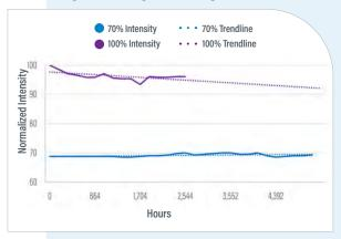
Figure 9. LED Degration Testing - VisiCure
