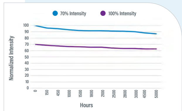
Figure 4. LED Degradation Testing - RediCure®
