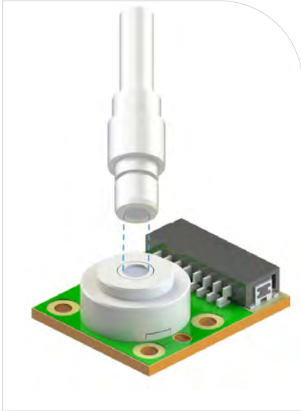
Figure 10. Aperture with 5-mm Lightguide
