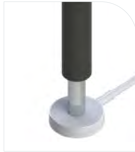
Figure 8. BlueWave® LED Prime Using a 8-mm Lightguide, Measured Directly on the Surface of the Radiometer
