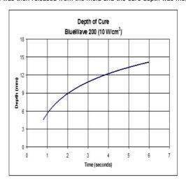
C At 53 mm [2.1 in] focal distance. Maximum speed of conveyor is 8.2 m/min [27 ft/min]. Intensity was measured over the UVA range (320-395 nm) using the Dymax ACCU-CAL™ 160 Radiometer.
