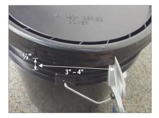
Figure 2. Place the Cutting Tool Under the Cover Skirt and Cut  $\frac{1}{2}$ " Slits from the Bottom Up, 3"-4" Apart
