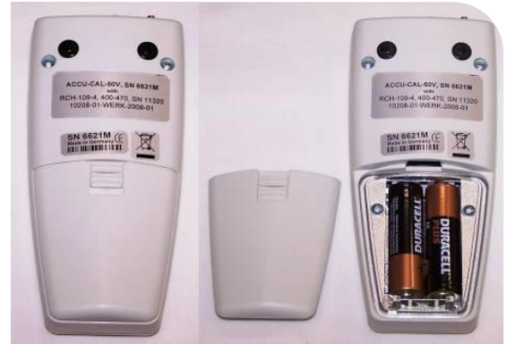
Figure 7. Battery Compartment (Closed & Open)
