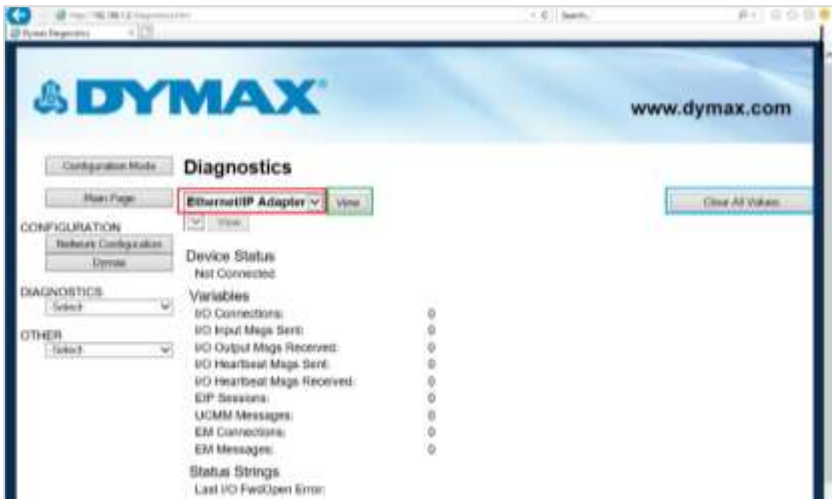
Figure 25. Diagnostics Page – Ethernet/IP Adapter
