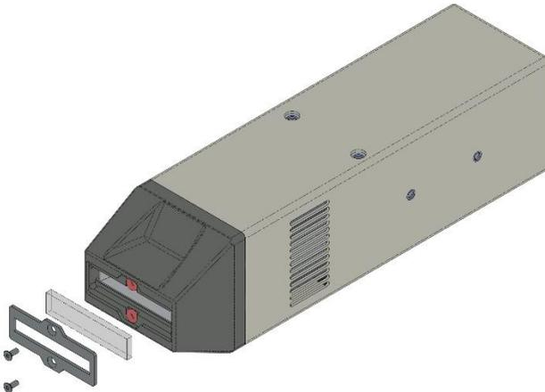
*NOTE: If the old window has shattered, be sure to remove all debris before attempting to install the new glass window.*
