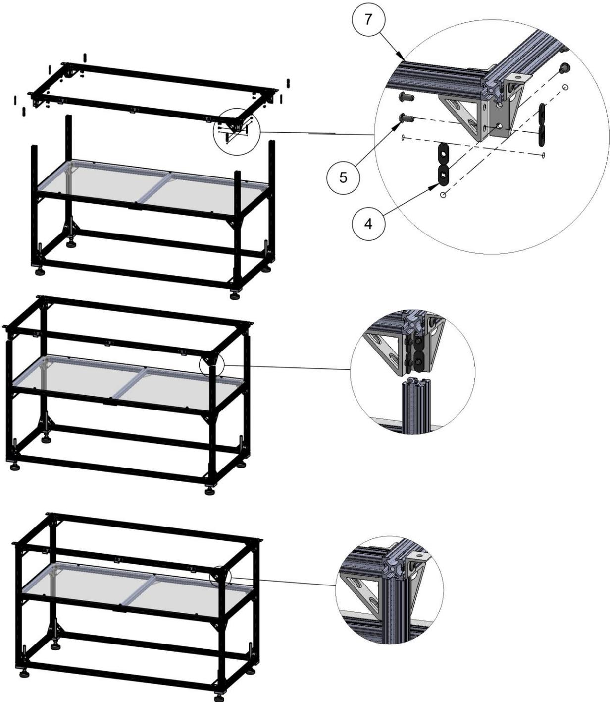
Figure 7. Attach Top Assembly
