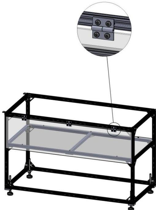
Figure 9. Door Assembly Attached
