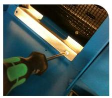
Figure 2. Installing Frame Tab
