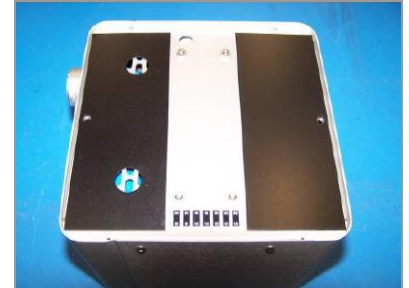
Figure 4. Two Temperature Control Plates Installed
