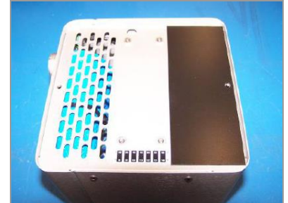
Figure 2. One Temperature Control Plate Installed
