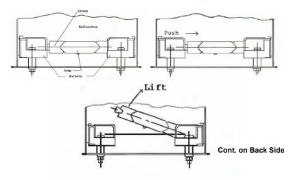
**CAUTION:** ALWAYS USE A SOFT, CLEAN RAG, CLEAN PAPER TOWEL OR GLOVES WHEN HANDLING THE LAMP. SKIN OILS LEFT ON THE LAMP WILL BURN INTO THE QUARTZ, REDUCING OUTPUT INTENSITY. IF THE LAMP IS INADVERTENTLY TOUCHED, CLEAN LAMP THOROUGHLY WITH A SOFT CLEAN RAG AND ALCOHOL. LAMP CONTAINS A SMALL AMOUNT OF MERCURY. DISPOSE OF ONLY ACCORDING TO ALL LOCAL, STATE, AND FEDERAL REQUIREMENTS.
