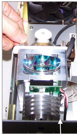
Figure 11. Tighten Mounting Bracket Thumbscrews
