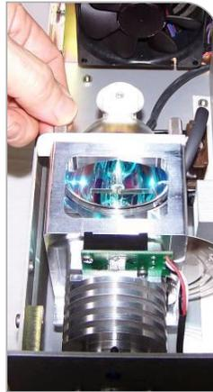
Figure 11. Tighten Mounting Bracket Thumbscrews
