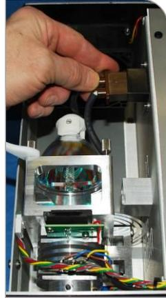
Figure 10. Plug in Bulb
