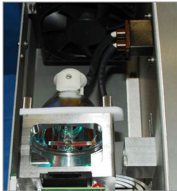
Figure 2. Bulb Installed in Bulb Mount
