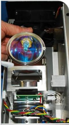
Figure 9. Install Bulb
