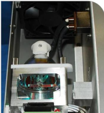
Figure 2. Bulb Installed in Bulb Mount
