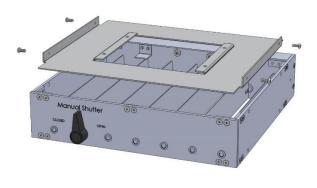
**Figure 4.** Flood Lamp with Adapter Plate Installed
