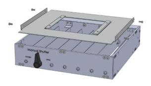
**Figure 13.**Remove the Filler Plate from the Lamp
