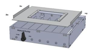
**Figure 7.** Attach the Mounting Plates to the Flood Lamp
