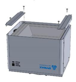
3. Install the assembly into the Manual Shutter and attach it with four 8-32 x %" screws removed in instruction one (Figure 8).
