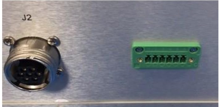
Figure 2. Additional 6-Pin Connector on the Rear Panel of the Power Supply Box
