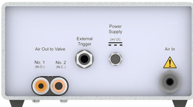
Figure 2. DVC-345 Component Diagram (Rear)
