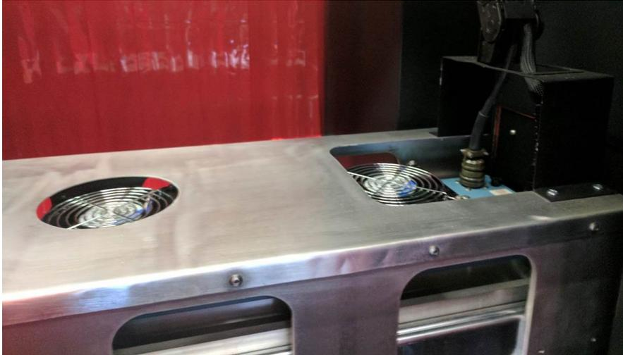
4. The curing chamber is surrounded by an enclosure, and has a perforated screen on top. Adjustable panels are located on the infeed and outfeed openings of the cure chamber area. Slide the panels up and down to allow for clearance of the parts being run, but low enough to reduce stray light emissions from these openings. There are two layers of light-blocking curtains (Figure 7 & Figure 8) after the entrance to the curing chamber and before the exit of the curing chamber.
