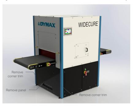
Figure 19. Remove Black Panel on Left Side of Conveyor
