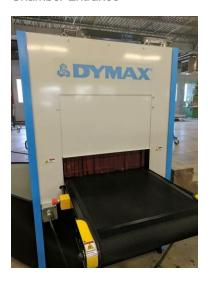
Figure 8. Light-Blocking Curtains in Curing Chamber (Top View)
