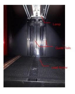
Figure 22. Guide Bars & Lead Screw (Close Up)
