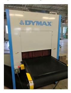
3. The irradiator is mounted on a linear stage that allows the height of the curing lamp to be adjusted from the conveyor belt. Use the control functions on the HMI to move the UV irradiator up or down as needed to allow for parts clearance and/or optimized cure height.
