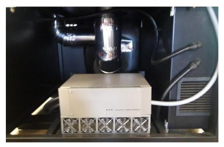
On the right side of the opening, towards the front of the conveyor, is a black-louvered fan cover. This cover can be removed by placing a flat-blade screw driver between the cover and the electrical housing and lifting the cover away from the housing (Figure 20).
