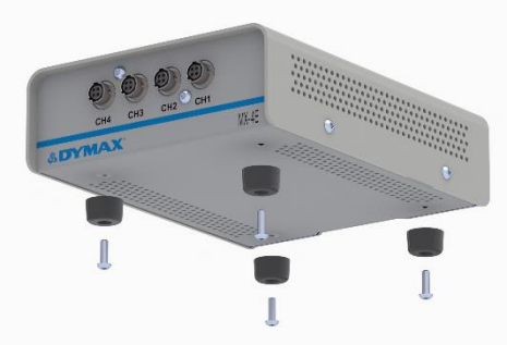
Figure 2. MX-4E Rubber Feet Installation
