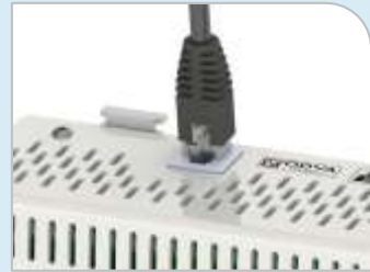
Figure 10. Shielded Ethernet Cable in RJ45 Port
