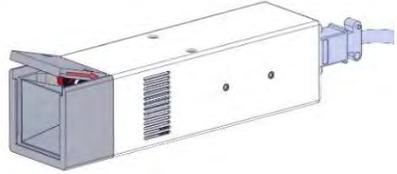
4. Slide the damaged glass cover out (Figure 6), taking care not to touch the metallic reflector surfaces.
