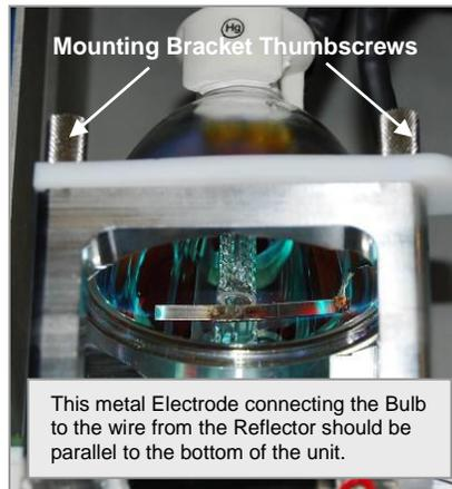
Figure 21. Bulb Electrode
