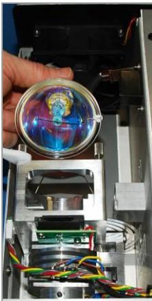
Figure 19. Install Bulb
