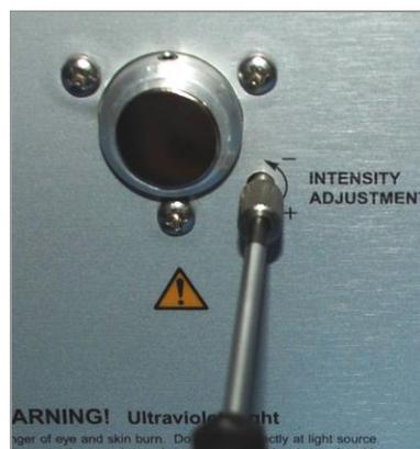
Figure 25. Intensity Adjustment Knob
