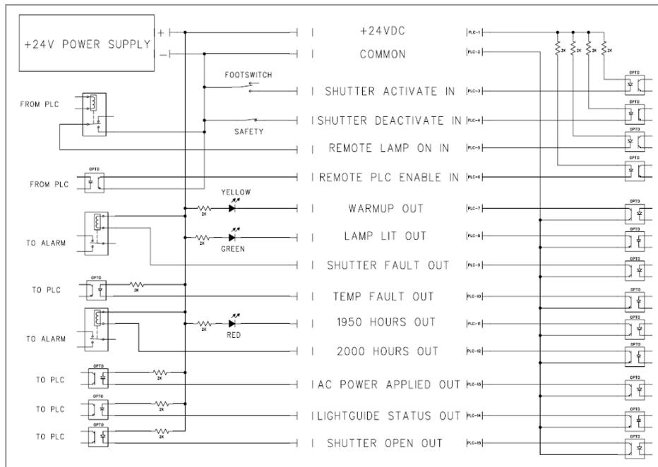
**Figure 27. 15-Pin I/O Signals**
