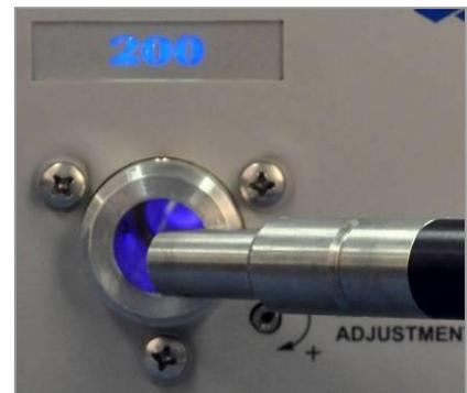
Figure 5. Insert Lightguide into Lightguide Mount
