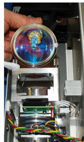
Figure 14. Remove Bulb from Bulb Mount
