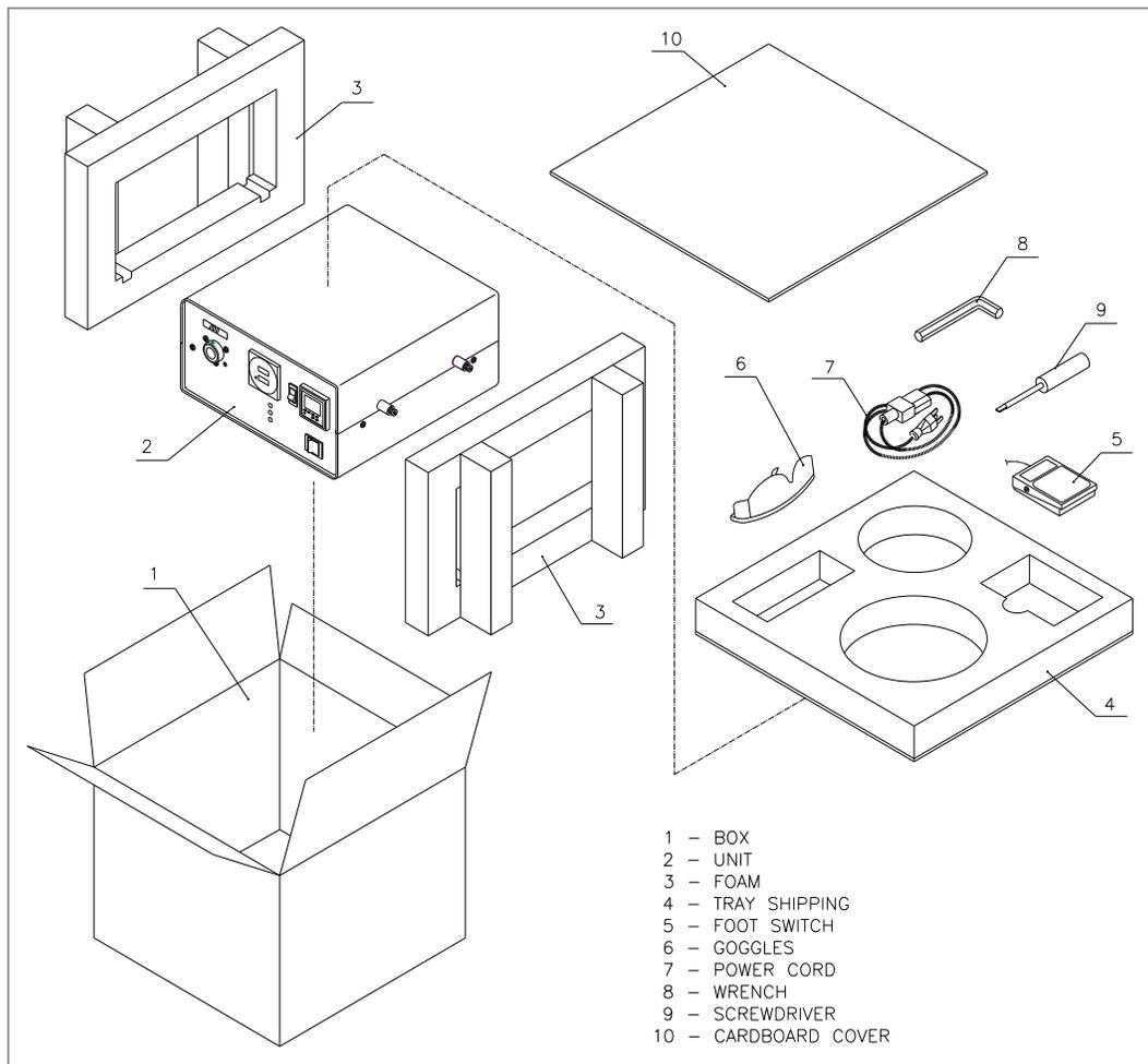
Figure 1. BlueWave® 200 (PN 40075 & PN 40080) Unpacking Diagram
