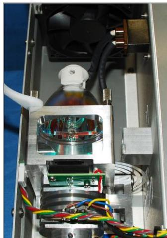
Figure 13. Lift Bulb Mounting Bracket
