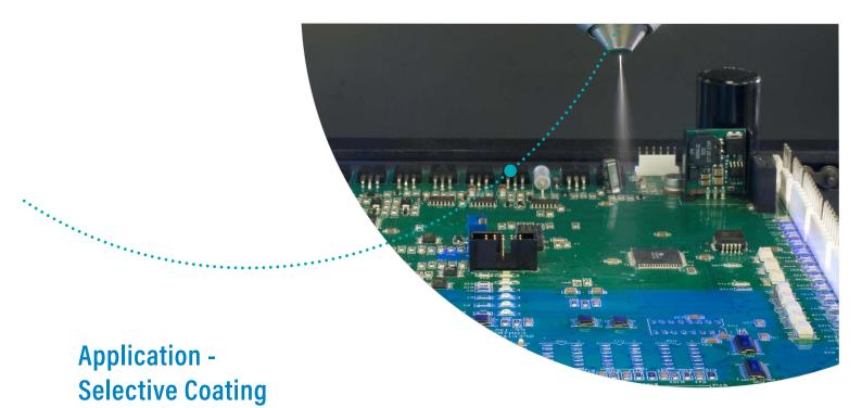
The effectiveness of a conformal coating is dependent upon how well it is applied. Conformal coatings can be applied using simple hand-application equipment, but are most commonly applied using three- or four-axis robotic selective-spray systems. This method allows for sufficient coverage of all areas that require coating while avoiding those areas that must not be coated.
