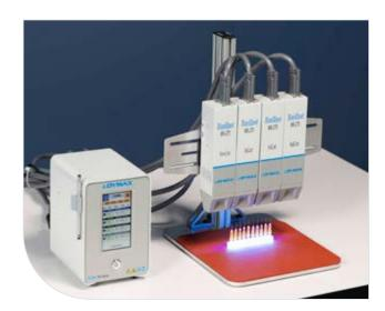
The BlueWave® MX-275 curing system is a high-intensity UV LED flood-curing system. Light energy is delivered in a line pattern instead of traditional patterns. A single BlueWave® MX-275 emitter provides a 5 mm x 50 mm curing area, but when paired with a multichannel controller, up to four emitters can be used to produce a curing area as large as 5 mm x 200 mm in line patterns.
