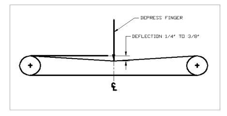
Dymax recommends that the ZIP Shutter's Curtain Drive-Belt's tension be checked at least once every three months. Follow the instructions below to check the Curtain Drive-Belt's tension.
