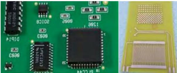
A humidity chamber was set to 85°C, 85% RH for 2,000 hours to evaluate heat and humidity resistance of the coatings. Salt spray corrosion resistance was evaluated using ASTM B117.
