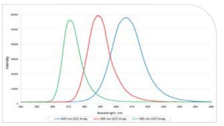
Example of a Light-Curing System Spectral Output Chart
