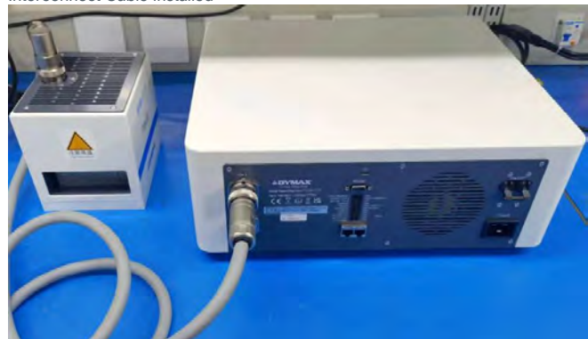
Figure 7. Interconnect Cable Installed
