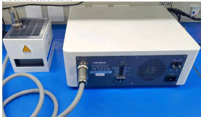
Figure 7. Interconnect Cable Installed
