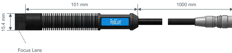
Figure 41. Focus Lens Dimensions
