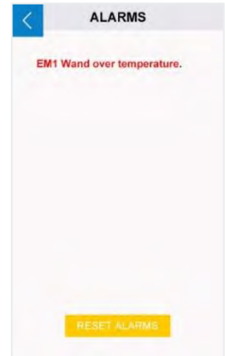
Figure 38. Temperature Alarm Screen
